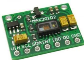
Figure 2. MAX30102 Heart Rate And O<sub>2</sub> Concentration Sensor
